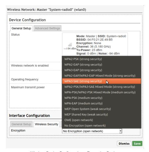
Wireless Device Configuration – Encryption Settings
