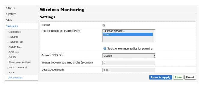
Scanning results can be obtained by a SNMP request. Getting queue entry from remote host
